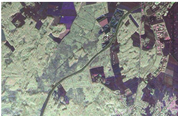
Figure 1 SAR image of forested region. Coloured composite of H- and V- channels, multi look image.
