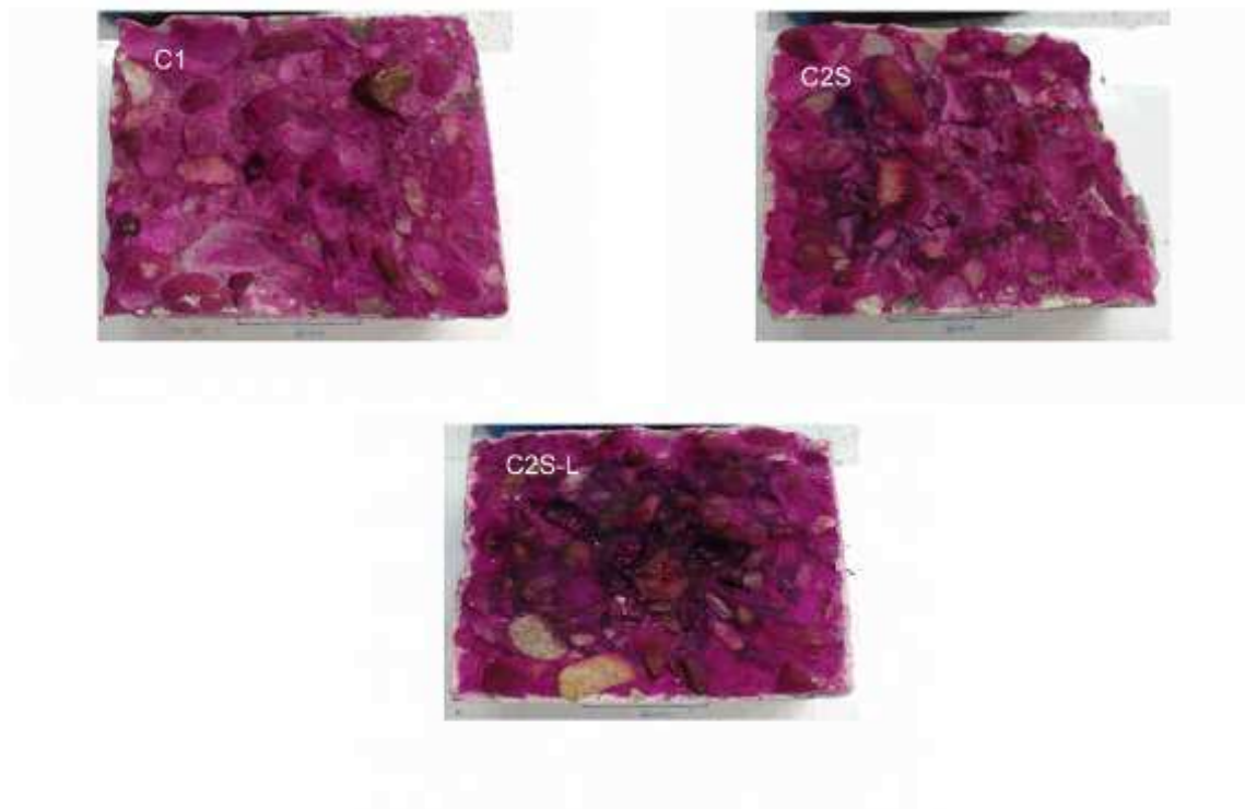
Figure 3 Extent of carbonation among the investigated concretes following conditioning at 20 °C and 65 % RH for 21 days as a function of cements: Mix C1, Mix C2S and Mix C2S-L
