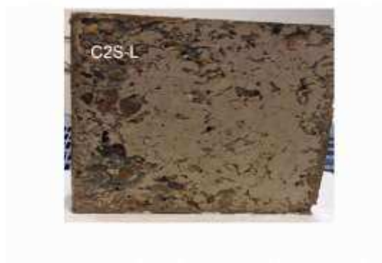
Figure 5 Evidence of freeze-thaw damage in concrete as a function of cement composition after 56 freeze-thaw cycles as a function of cements: Mix C1, Mix C2S and Mix C2S-L
