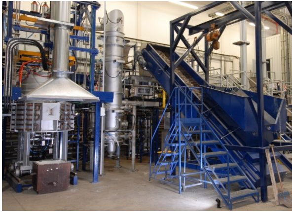
Figure 11: Direct photo of major components of the pilot plant: two-stage fluidised bed and plasma converter for syngas generation (left), syngas storage vessels and bio-SNG facility (right).
