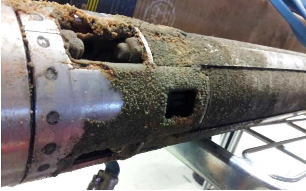
Figure 4. Photograph illustrating the presence of precipitates on the water sampling pump recovered from monitoring well HN-04 on the 13 th of August 2013. The diameter of the pump is 101 mm.
