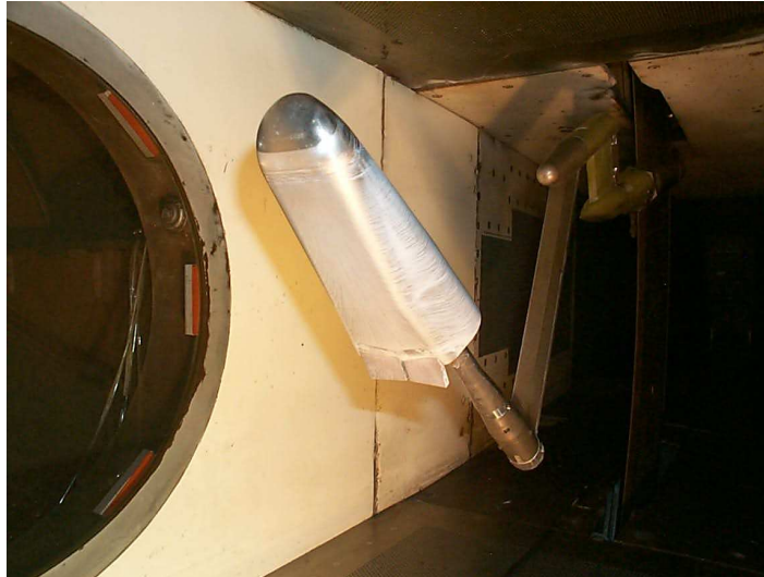
Figure 3 : Pre-X configuration with Wind Tunnel support at 15° flap deflection angle
