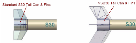
Fig. 13: Modification of 1st Tailcan Assembly
