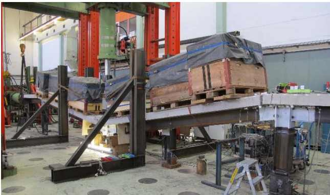
Fig. 3: Deformed 2D frame test FT 2.
