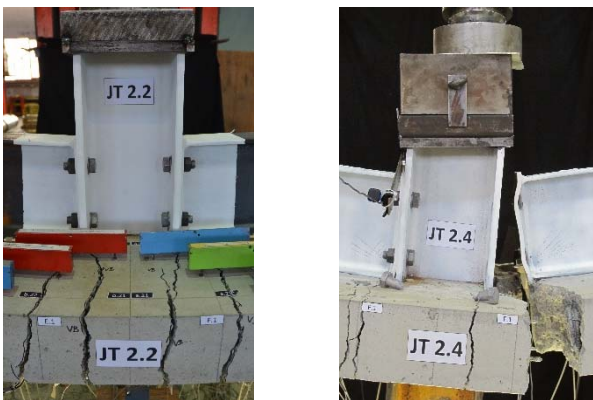
Fig. 2: Negative moment joint tests.
