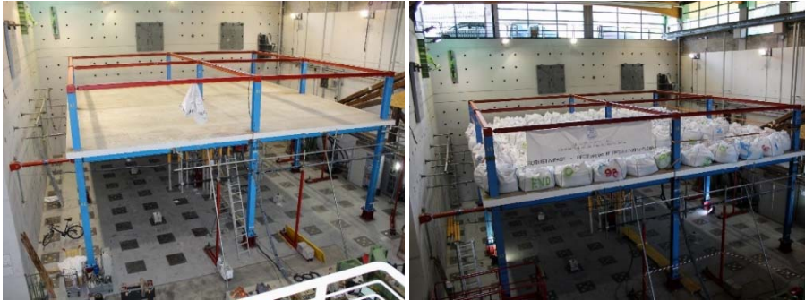
Fig. 11: The specimen of the symmetric frame.
