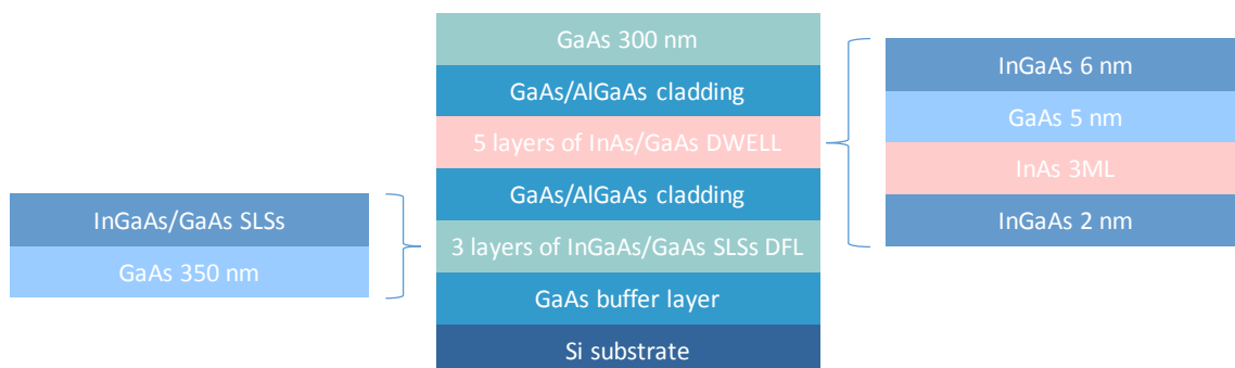
Figure 1. Schematic diagram of InAs/GaAs QD structures grown on a Si substrate.
