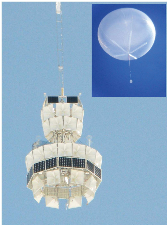
FIG. 1 (color). The ANITA-II payload on ascent with the lower eight horn antennas deployed. The payload height is \sim 8 \text{ m} , and each antenna face is 0.95 \text{ m} across. The inset shows the balloon and payload viewed telescopically at float altitude of 35 km.
