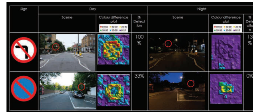
▲ Figure 8. The colour difference of signs under daytime and night-time scene, shown through a surface plot
