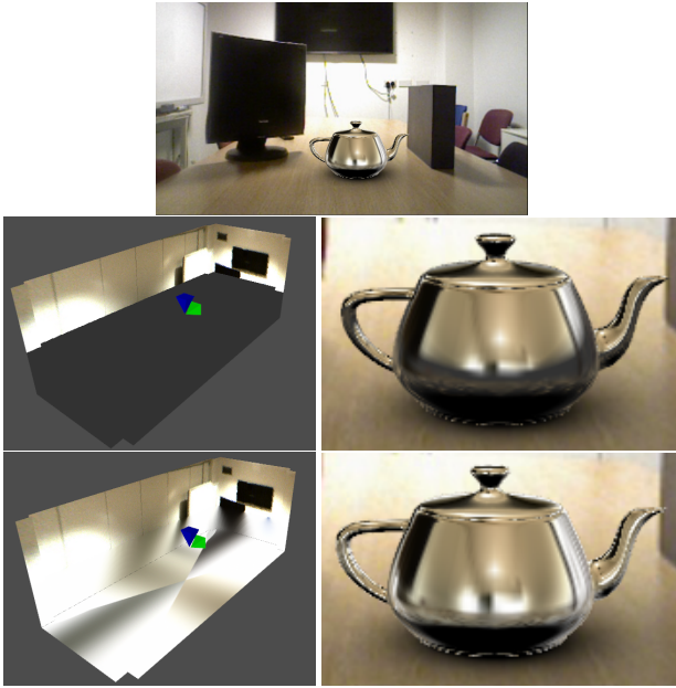
Figure 5: Scene containing a virtual teapot, with and without inpainting applied. Top: augmented image (with inpainting). Middle: view of coarse model and closeup of teapot, without inpainting. Bottom: view of coarse model and closeup of teapot (with inpainting).
