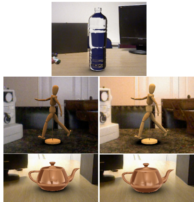
Figure 7: Examples of some of the other virtual objects that can be simulated using environment maps. Top: Water bottle, simulating refraction of the environment. Middle: Wooden mannequin, simulating diffuse shadowing, reacts to a ceiling light being turned on. Bottom: Metallic teapots, simulating different levels of surface roughness.
