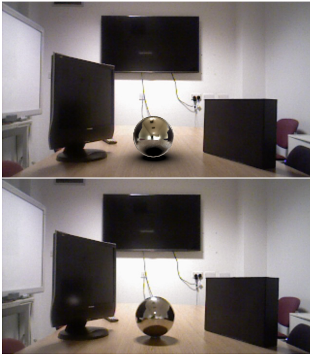
Figure 11: Comparison between a virtual reflective sphere and a real chrome sphere. Top: virtual sphere. Bottom: real sphere.
