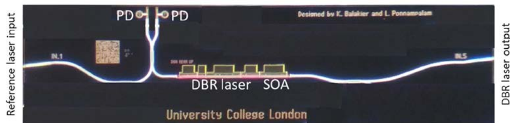
Fig. 2. Photographs of OPLL PIC with dimensions of 2 \text{ mm} \times 6 \text{ mm} . All components that do not form part of the OPLL are greyed out, so that the laser and photodiodes used in this experiment are more clearly visible.
