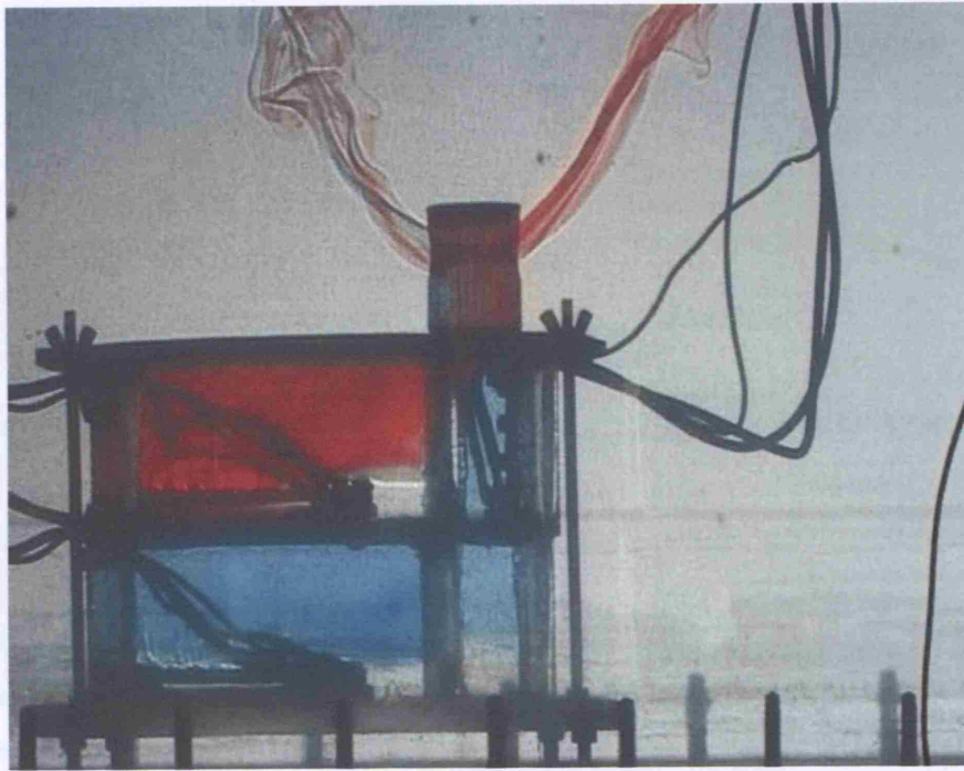
Figure 67: Simplified model sub merged in a water bath for simulation (Source: Lomas et al., 2008b)
