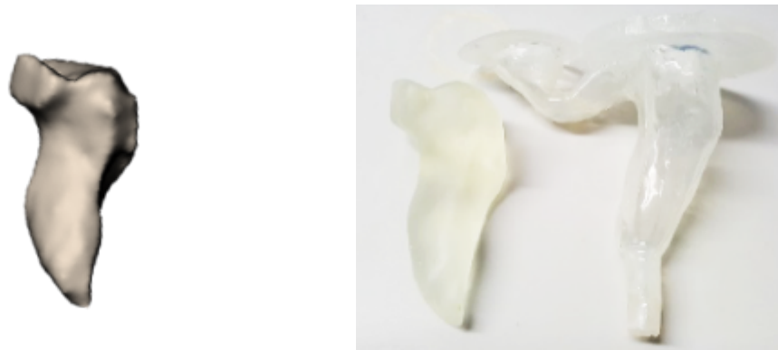
Figure 8.2: Human left ventricle ( left ) computerised Tomographic (CT) scan in its fully contracted state ( right ) left : mould to make ventricle sac right : silicon ventricle sac formed using mould.
