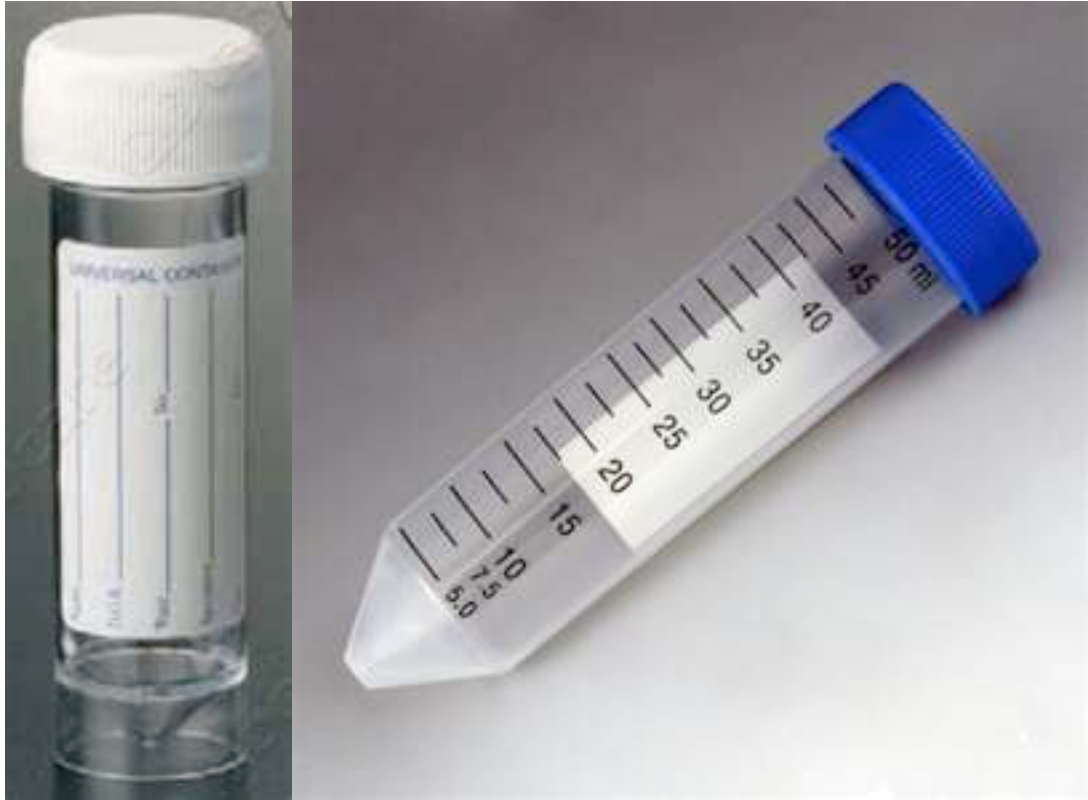
Photograph two: Left a polystyrene tube, which is more clear in appearance. Right, a polypropylene tube which appears more cloudy. Photos taken from www.djblabcare.co.uk
