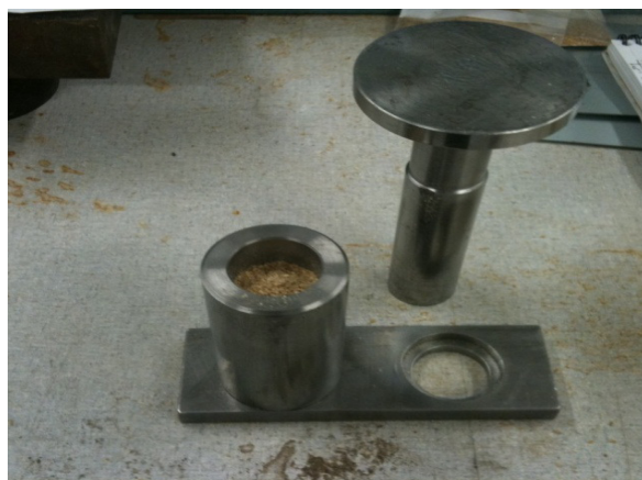
Figure 10: Blend of rice husks and corn cobs loaded into the 32 mm diameter mold
