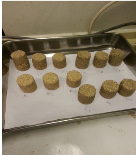
Figure 17: Briquettes produced from blends of rice husks, corn cobs and bagasse with different binders
