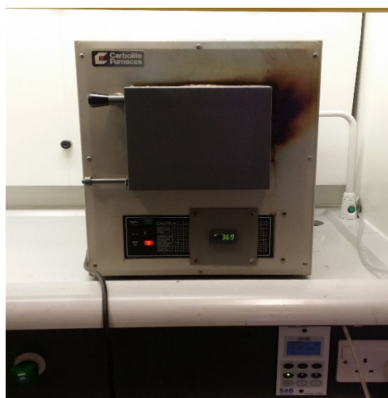
Figure 19: Determination of ash content of briquettes produced with starch, biosolids and microalgae binders in a muffle furnace
