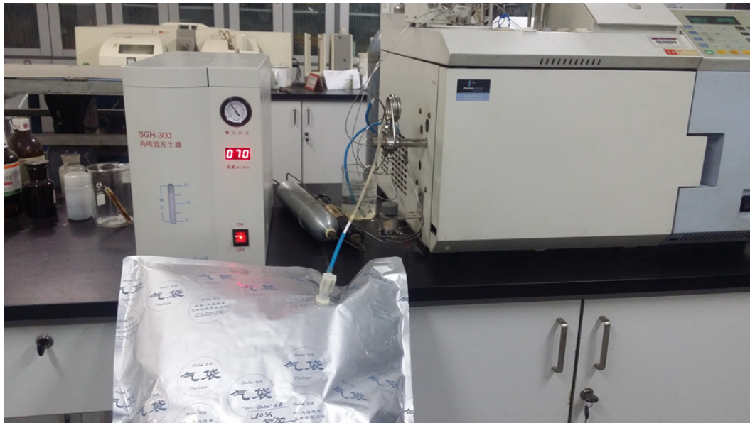
Figure 47: Analysis of gasification product gas using GCMS
