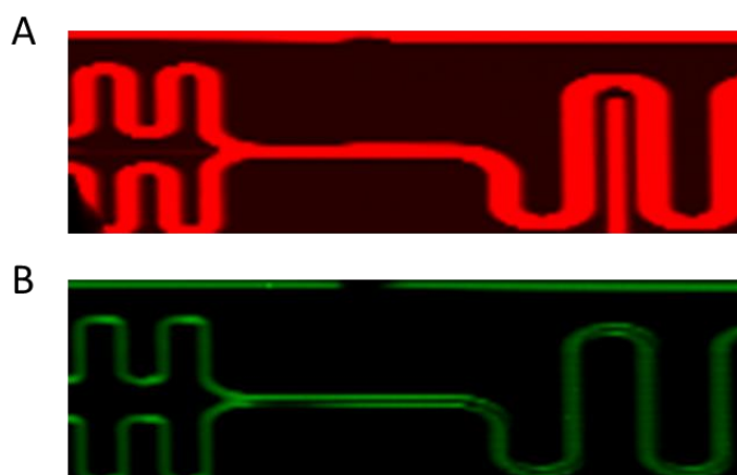
Figure 14. A) I_t map of the Si/glass micro-reactor zoomed in to the mixture region in the channel and B) Pt XRF map (green) indicating laminar flow through the Si/glass micro-reactor. (Pt solution and H 2 O used as the reagents).
