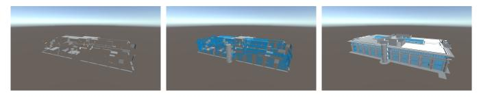
Figure 1: Test scene used in our measurements being dynamically loaded from a remote version controlled repository using a newly developed 3DRepo4Unity library. The building consists of 13k components and 4m vertices. Model courtesy of Skanska.
