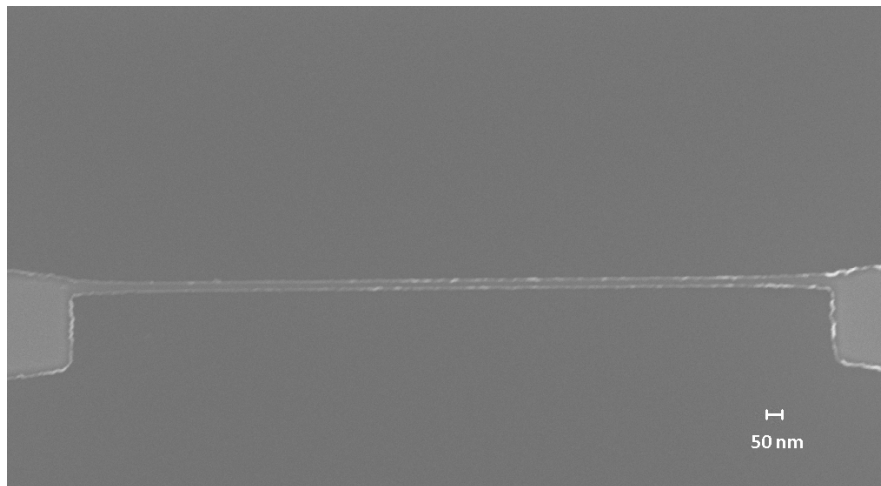
FIGURE 3.18: Reduced lilypadding on a 60 nm nanowire created with a resist layer 100 nm thick.
