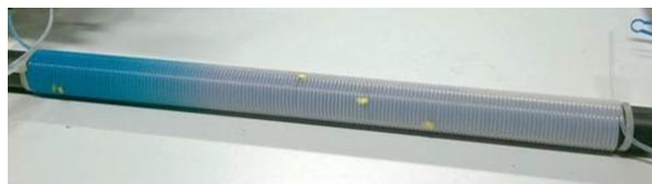
Figure 7.9. HCT constructed. PFA capillary 1 mm ID and 1.58 mm OD. External diameter of the coil structure = 17 mm. Number of turns = 80. \lambda=17.8 .
