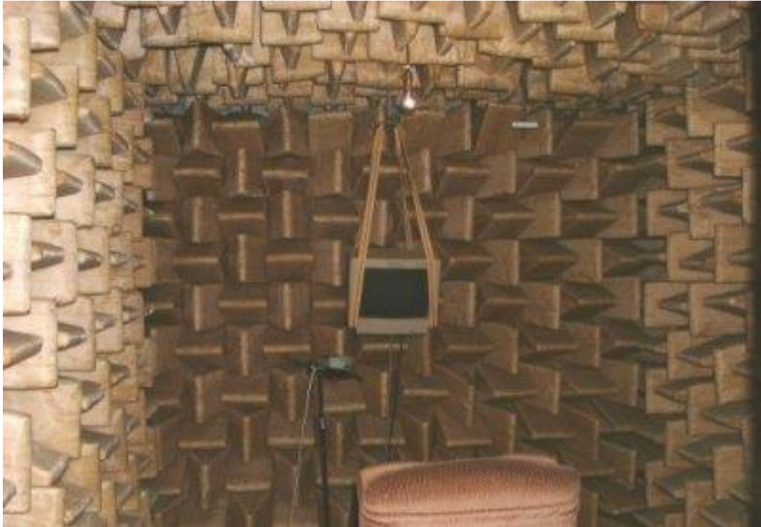
Photo. 1: The anechoic chamber
