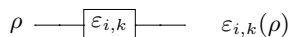
FIG. 5: Channel Building Block The building block effectively implements a quantum channel \varepsilon_{i,k} on the input state \rho where i refers the measurement bases and k the measurement outcome.
