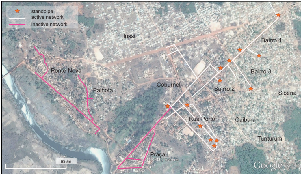
Figure 4. Bafatá piped water network: mains and standpipes in 2014 (Source: produced by authors based on information collected from ASPAAB and TESE)
