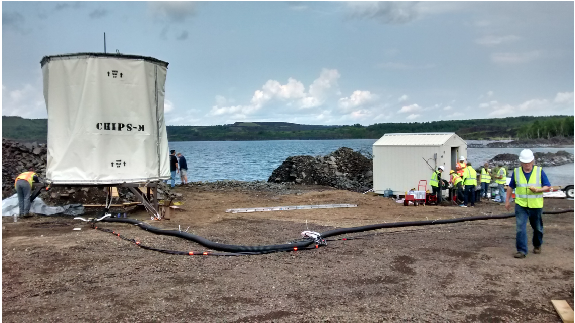
Figure 11.2: Photograph of the CHIPS-M prototype detector at the end of July 2014, shortly before deployment. Also pictured is the large umbilical cable carrying pipes from the detector to the small building housing the water filtration system, and the smaller black cables that provide power and communication to the DOMs.
