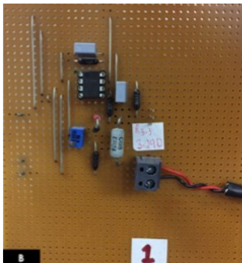
Figure 2-10 (A) Sensor heating unit for the eight sensors used in this system. (B) Close up of an individual heating board responsible for heating the sensor in port 1.
