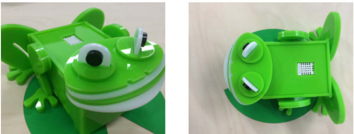
Figure 37. The Frogbox temperature and humidity sensor sitting on a cardboard Lilly pad.
