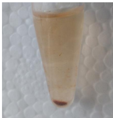
Figure 4.4.7.4. Macro image of the resulting MTX.IONP produced via ligand exchange in water. The resulting material was insoluble in a range of organic and polar solvents making it unsuitable for downstream applications.
