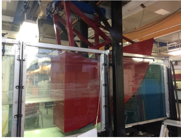
Figure 16 Piston wave paddle in the 13.4m wave flume
