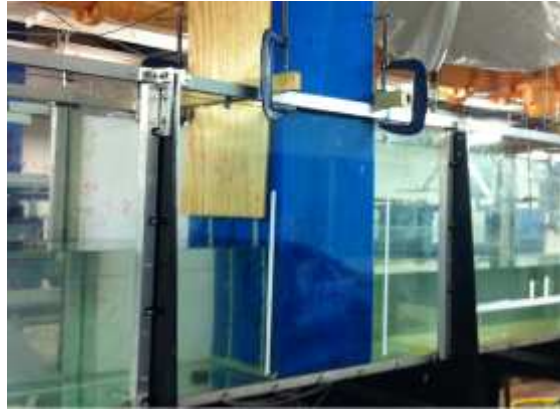
Figure 60 Picture of steady flow experiments through the porous foam dam
