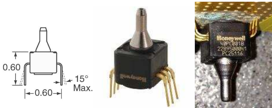
Figure 25 40PC Series Honeywell pressure transducer and their power supplier used
