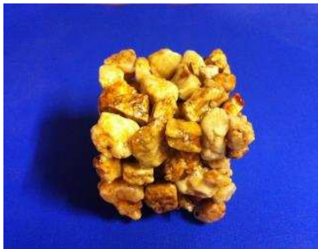
Figure 188 Sample of gravel bonded with Elastocoast
