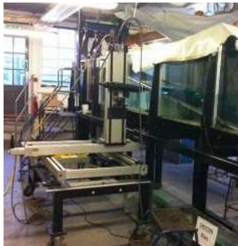
Figure 52 Picture 3-axis TSI traverse
