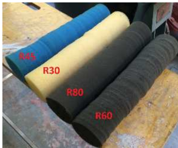
Figure 186 Cylindrical foams used for constant head tests
