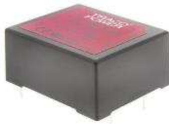
Figure 25 40PC Series Honeywell pressure transducer and their power supplier used
