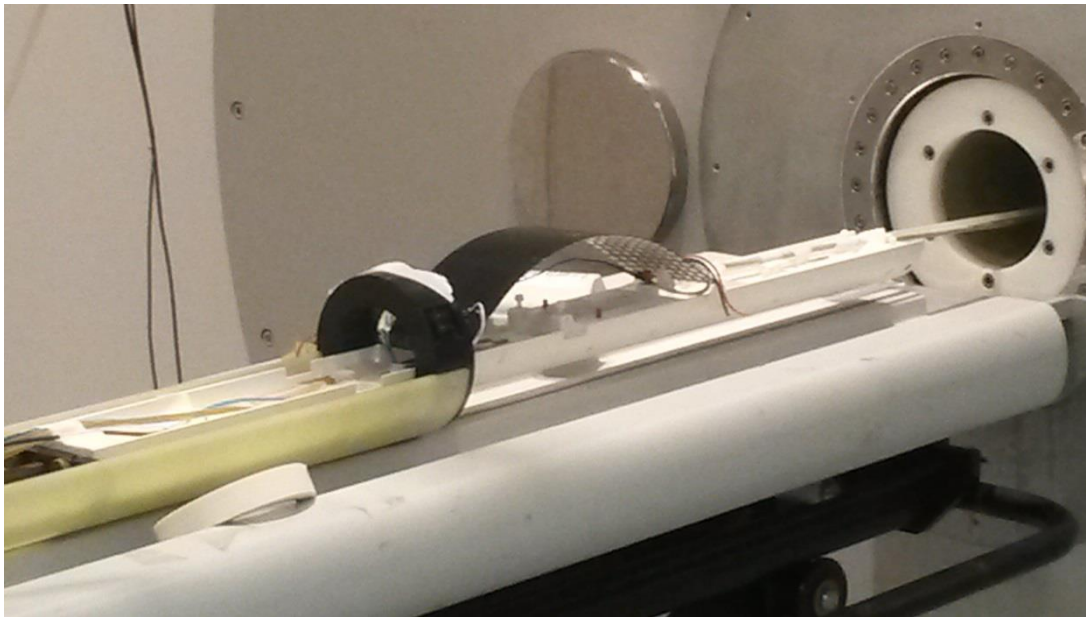
Figure 4.17. Placement of LED board over the mouse cradle, for visual stimulation.
