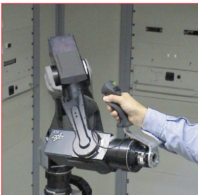
Lightweight robot as force-reflecting interface for virtual operating elements ■
