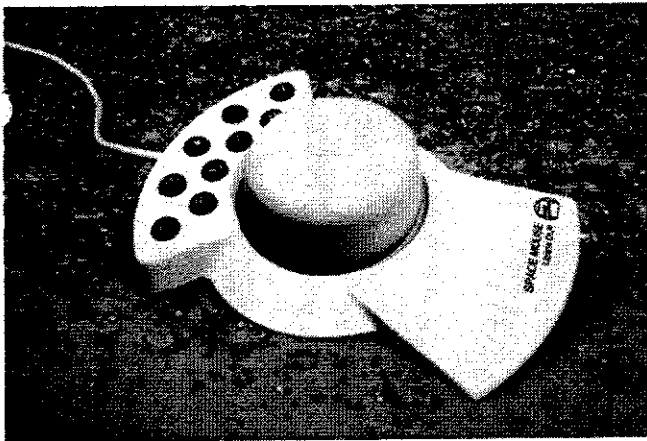
Fig. 27. Space Mouse (in USA and Asia called Magellan by our license partner Logitech).
