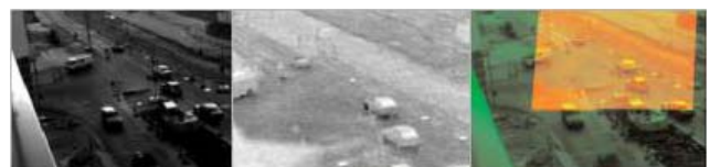
Figure 3: Sensor fusion of VIS and IR images (I)
