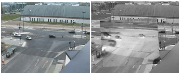
Figure 4: Sensor fusion of VIS and IR images (II)
