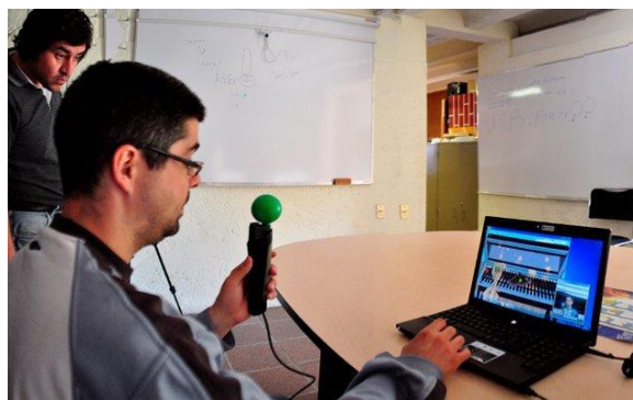
Fig. 1. The Gesture Therapy platform. One of the researchers is illustrating the use of it. The gripper, hold with the left hand here, serves to control an avatar on the virtual scenario. 3D location of the hand and gripping pressure are sensed and send to the computer for further processing.
