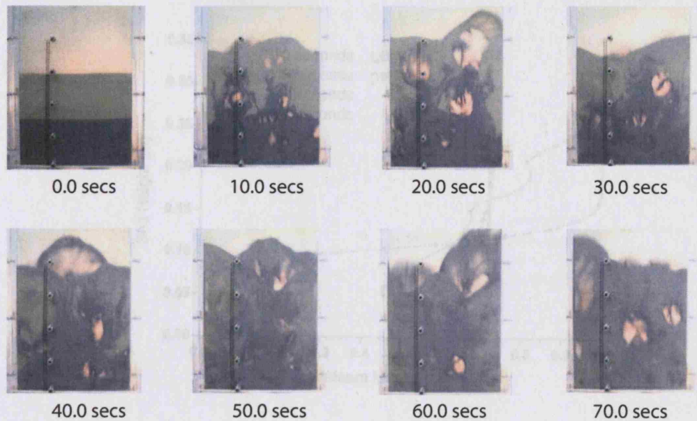
Figure 6.14: Experimental snapshots of the fluidized bed using a mixture fraction of 0.50 jetsam at an excess gas velocity of 0.20m/s.
