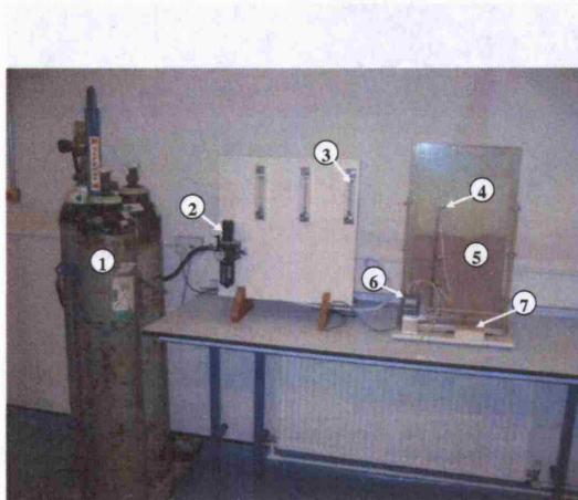
Figure 3.24: 2D Experimental vessel: 350 mm wide, 600 mm height, 10 mm depth
