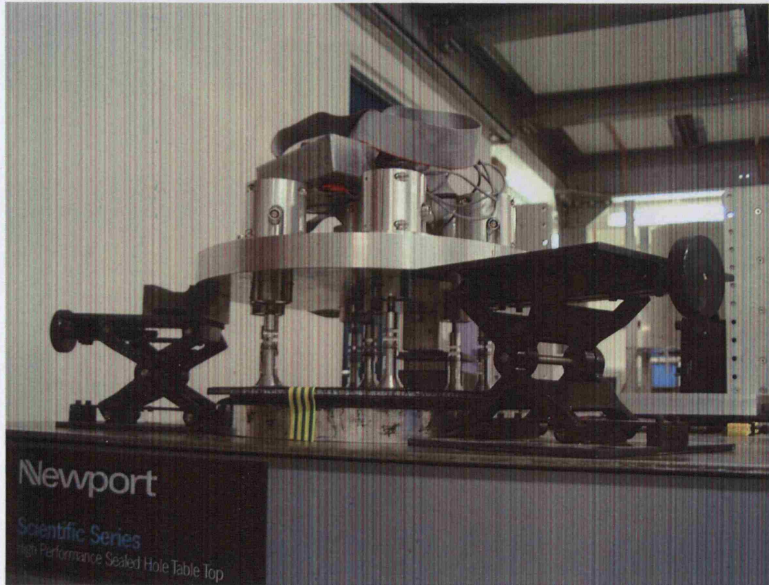
Figure 4.4: Picture of the gluing rig used to assemble the mirror systems. The raised stages stop the backing plate from stressing the faceplate during the cure process. The picture also shows the actuator mounts and flexures.
