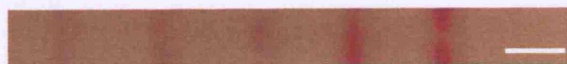
Figure 3.26: OTS/SiO 2 charge-written in tapping mode. KFM image of a detail of 5 lines charge-written in tapping mode at 10 \mu\text{m/s} tip velocity applying - 80 V voltages pulses at a 50 Hz rate. Scale bar = 3 \mu\text{m} , scale range = 10 V.
