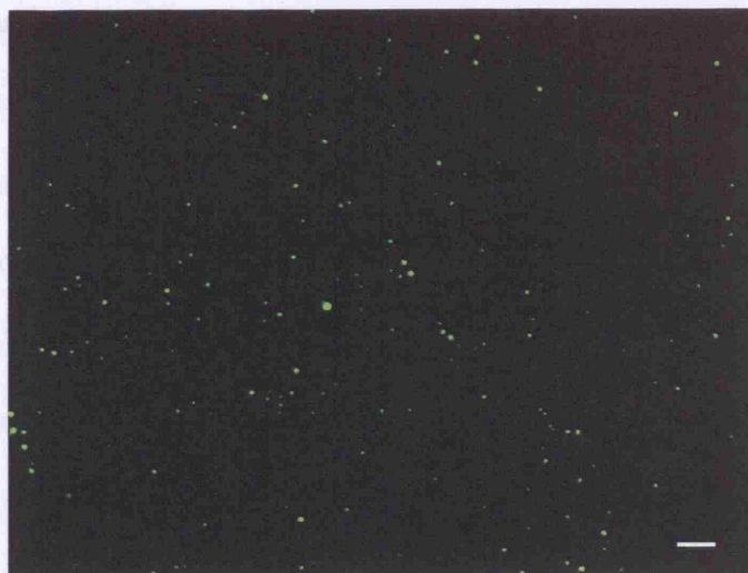
Figure 4.14: Avidin Fluorescein Emulsion. Fluorescence image using an inverted light microscope (Olympus IX71, Middlesex, UK) with the 40x, NA 0.60 objective. The excitation/emission wavelengths of the FITC fluorophore was 490 nm/520 nm. Filters used to image the fluorescence emission: excitation filter: 460-490 nm, emission filter: 520 nm, dichromatic filter: 500 nm. The fluorescence image was recorded using a ORCA-ER digital camera (Hamamatsu, Welwyn Garden City, UK). Scale bar = 10 \mu\text{m}
