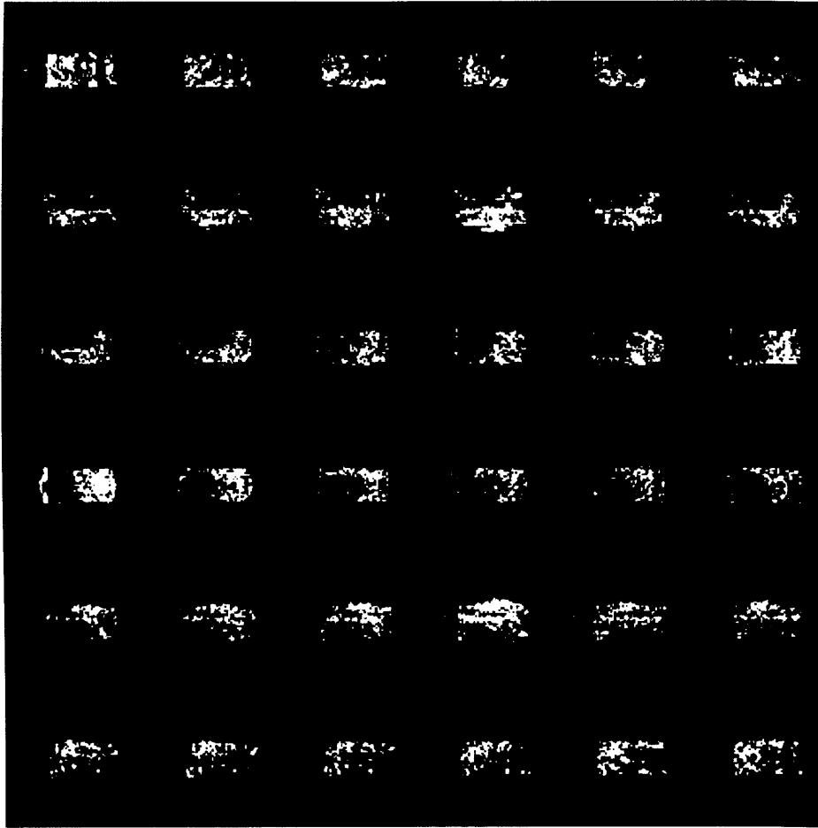
Figure 71: Changes in the HH polarimetric intensity at 10^\circ intervals over a complete revolution (MBT Imaged at 41^\circ grazing processed at 20cm range and azimuth resolution)
