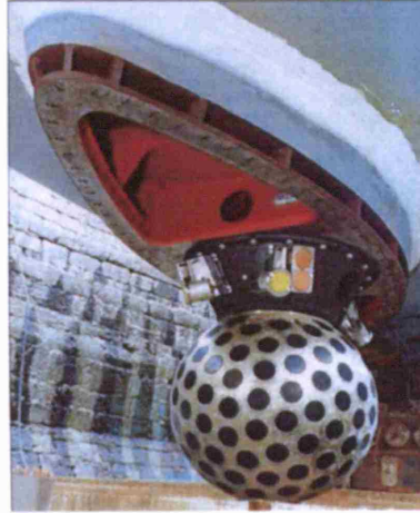
Figure 1.3: A spherical array for a SONAR application. SONAR works with acoustic waves, so that the pattern from a SONAR array can be described with scalar functions. Although the velocity of sound is much slower than the propagation velocity of an electromagnetic wave, the used wavelengths are often comparable. The size of the array of pressure sensors shown above is therefore representative for what could be expected to be the size of a spherical antenna array for RADAR applications. Courtesy of Thales
