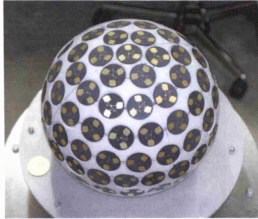
Figure 1.2: A small spherical array demonstrator, as presented in [24]. It is interesting to note that without mutual awareness, their design approach for the subarrays has converged to a solution that is very similar to the design of our prototype spherical array. Illustration used with kind permission from Dr. Peter Knott from the Research Institute for High Frequency Physics and Radar (FGAN-FHR) in Germany.
