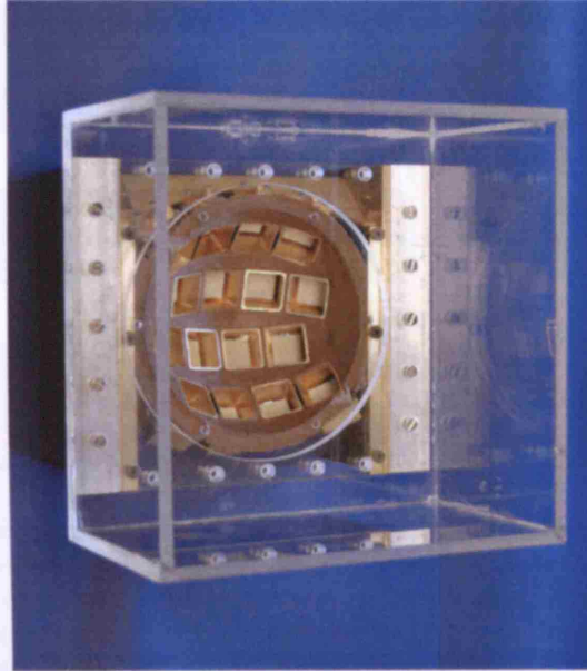
Figure 1.5: A concave spherical array prototype for breast cancer detection. Illustration used with kind permission from Dr. Ian Craddock from the Dept. Electrical & Electronic Engineering of the University of Bristol.
