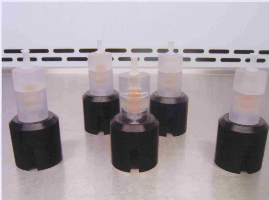
Figure 7.3 Bases for the chambers were made from black Delrin (upper), the in-vitro chambers were supported on bases allowing tube access to the underside luer port (lower). Dimensions in mm.
