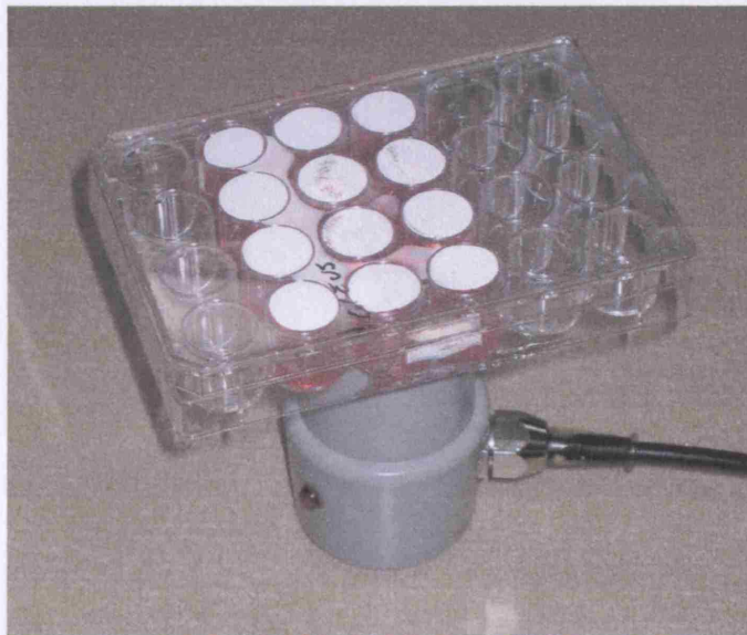
Figure 2.10 The application of Ultrasound to the cytoball experiment plate using a coupling gel.
