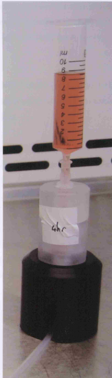
Figure 2.8 The in-vitro TNP pump fully assembled with upper inverted media containing syringe and lower suction tubing.
