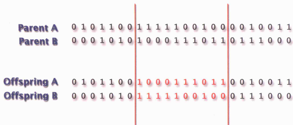
Figure 1.7: A two-point crossover operator is shown. Two points along the chromosome are selected at random and the region spanning these two positions are exchanged between parents to produce new offspring.
