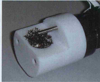
Fig 4.6 A piece of foam in the Evaporimeter probe chamber.
