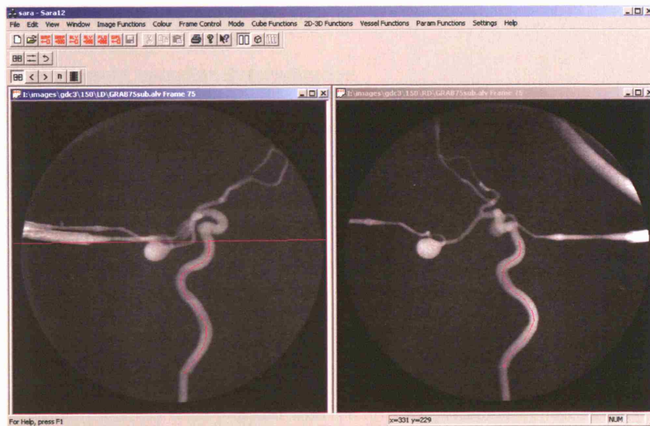
Figure 6.32: SARA 2000 software: Stage 3: 2D Vessel Centreline Determination: The rough centreline, shown in purple, is defined using the epipolar constraint.
