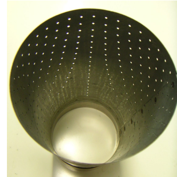
Figure 3. Photo of the perforated end diffuser
