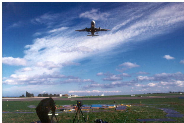
Fig. 1 Microphone array installed on the test site
