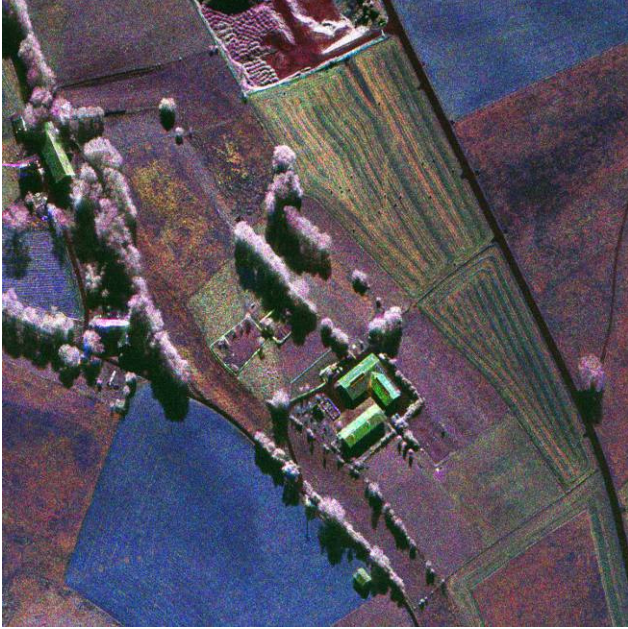
Figure 7 Zoom into an F-SAR quad-pol X-band image. Spatial resolution 0.4m. Site: Kaufbeuren, Germany.
