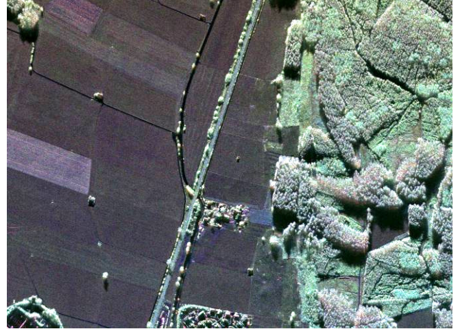
Figure 9 Zoom into an F-SAR quad-pol S-band image. Spatial resolution 0.5m. Site: Kaufbeuren, Germany.
