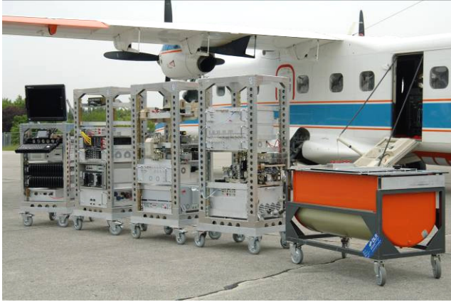
Figure 5 F-SAR X-C-S-band system prior to installation onboard DO228 aircraft for flight testing.
