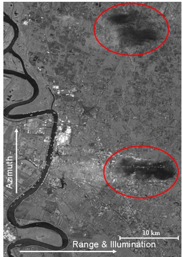
Fig. 6. A test case showing a comparison of X-band TerraSAR-X data and weather radar data (Nexrad, NOAA) acquired nearly simultaneously (within the same minute) over a scene close to New Orleans, US. A good agreement between the rain-cell signatures in the SAR image (right hand side) and the weather radar image (left hand side) can be observed. The effects are most pronounced for reflectivities of up to 50 dBZ.
