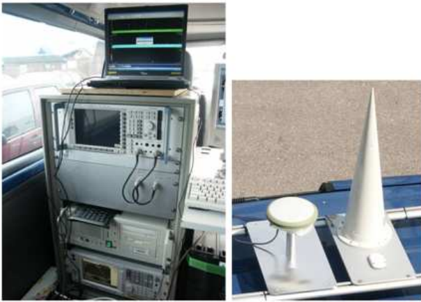
Fig. 1. Left: Measurement equipment in 19" from top to bottom: 1) Laptop with control software for Agilent PSA, 2) R&S FSH6, 3) Amplification and control unit by Joanneum Research, 4) Control and storage PC for the Joanneum Research unit, 5) Agilent PSA E4443A Right: Conical hemispherical antenna for interference measurements and two GPS-antennas
