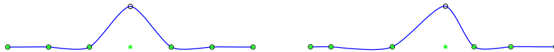
Fig. 3.3 Basis function of the NULI 4-point scheme with uniform knots (left) and non-uniform knots (right). The edge parameters are set to \lambda_i^0 = \frac{1}{2}, \forall i .
