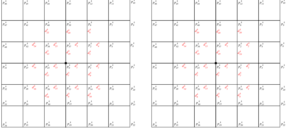
Figure 3: Left: indexing of points and parameters at refinement level k . Right: configuration of parameters in the tensor-product case.
