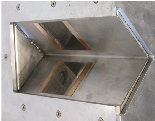
Fig.4: Bottom view of the lead housing. This is the mouse hole. Detectors face at 90°.
